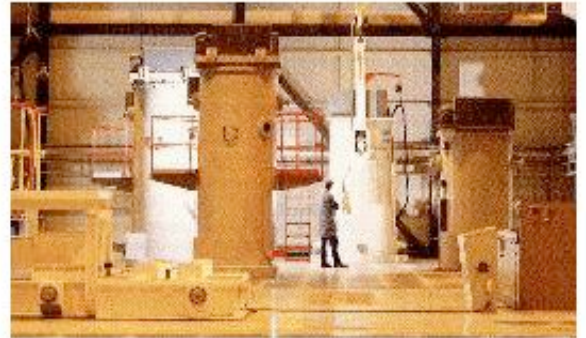
Figure 4: VHLW storage in air-cooled vaults
